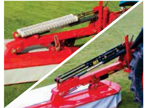
⑤ Mechanical or hydraulic relief - Vari Float
