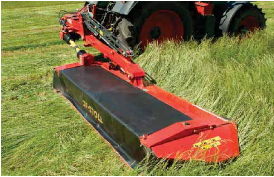
⑤ Mechanical or hydraulic relief - Vari Float
